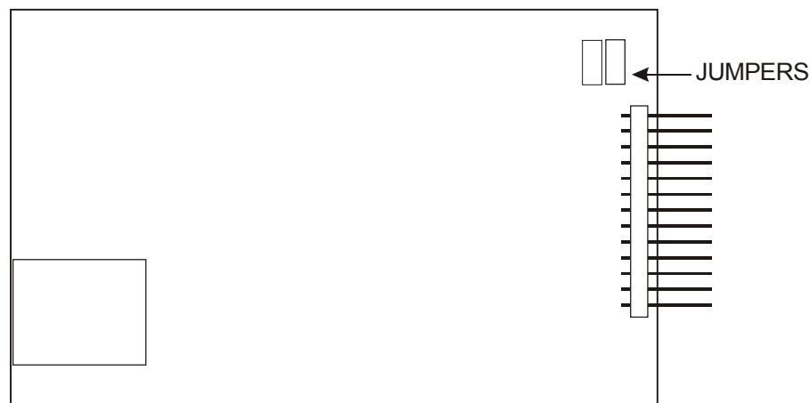
Figure C-4 ISDN Module processor setting jumpers
